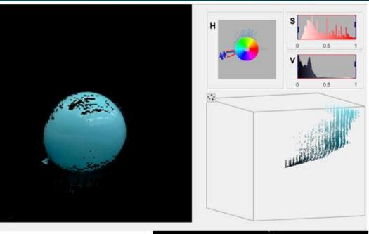
Reflected light can confuse the robot, this additional noise needs to be filtered out with morphological processing in order for the robot to correctly track the correct object.
